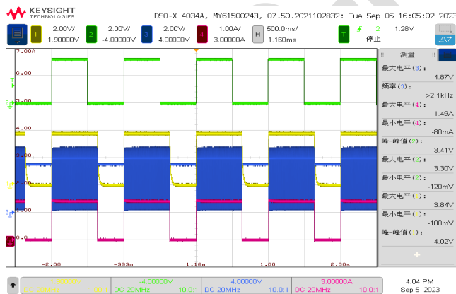
Fig-13: V_{IN}=3.6V , I_{LED}=1.5A , f_{STROBE}=1Hz , Flash time out = 600ms.
