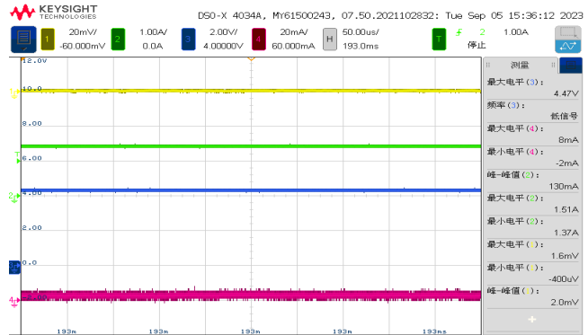
Fig-10: V_{IN}=3V (Pass mode). CH1- V_{OUT}/AC , CH2- I_L , CH3- V_{SW} , CH4- I_{LED}/AC
