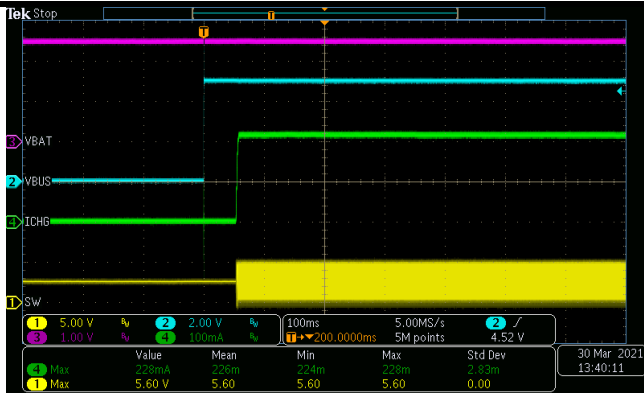
Figure 7. V_{BAT}=2.5V , plug in 5V VBUS CH1-SW, CH2-V BUS , CH3-V BAT , CH4-ICHG
