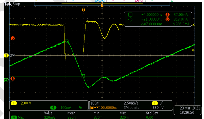
Figure 29. V_{BUS}=5V , ZCD: 32mA CH1-SW, CH4- I_L
