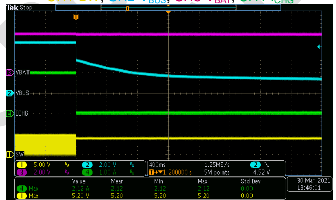
Figure 10. V_{BAT}=3.8V , plug out 5V VBUS CH1-SW, CH2-V BUS , CH3-V BAT , CH4-ICHG
