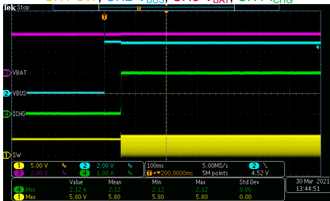
Figure 9. V_{BAT}=3.8V , plug in 5V VBUS CH1-SW, CH2-V BUS , CH3-V BAT , CH4-ICHG
